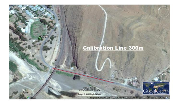
Overall calibration distance is 300 meters. Both ends are nailed with washers.
